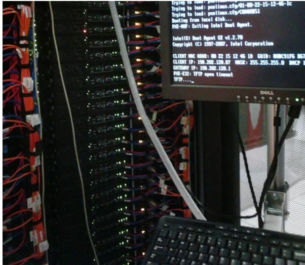
Figure 1.4: A rack for cluster with capacity for 60 mother boards.
