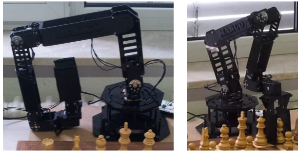
(a) The robot’s rest configuration (b) Picking up a piece close to its base
